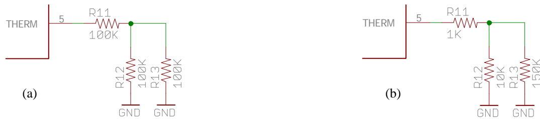
Figure 3-3. Comparison between the Version 1 THERM resistor values (a) and the datasheet values (b).
