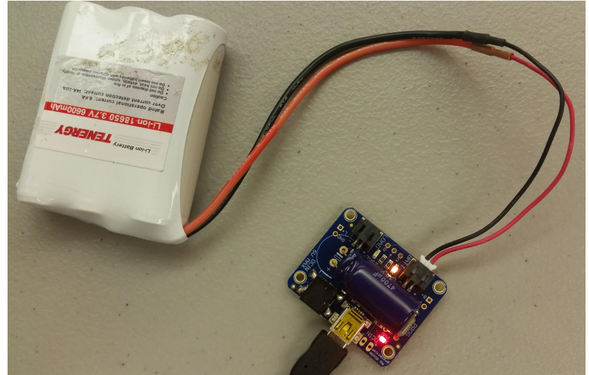
Charging Circuit (MCP73871 with Tenergy 18650 3.7V 6600mAh)
