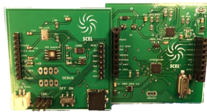
Figure 1-2. The Cranberry weatherbox – Third generation SCEL environmental sensor module.
