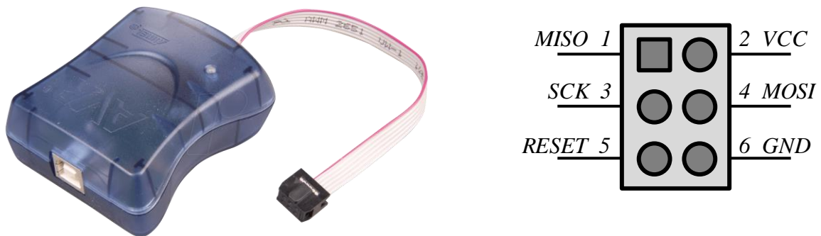
Figure 2-5. AVRISP MkII programmer and the ISP interface.
