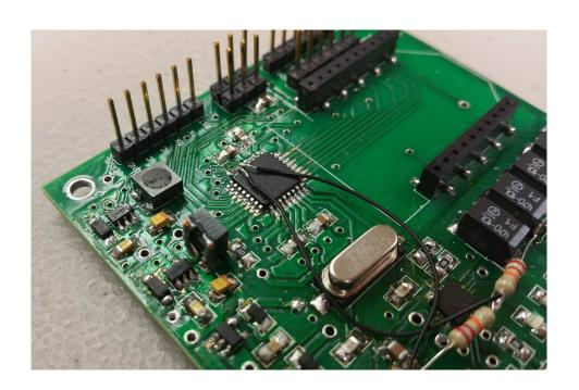
Incompatible inductor (DCR) for 5V boost converter
