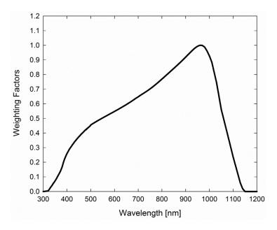
Spectral response estimate of Apogee silicon-cell pyranometers. Spectral response was estimated by multiplying the spectral response of the photodiode, diffuser, and adhesive. Spectral response measurements of diffuser and adhesive were made with a spectrometer, and spectral response data for the photodiode were obtained from the manufacturer.
