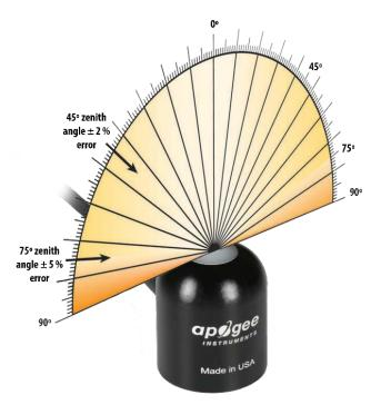
Directional, or cosine, response is defined as the measurement error at a specific angle of radiation incidence. Error for Apogee siliconcell pyranometers is approximately  $\pm 2\%$  and  $\pm 5\%$  at solar zenith angles of 45° and 75°, respectively.
